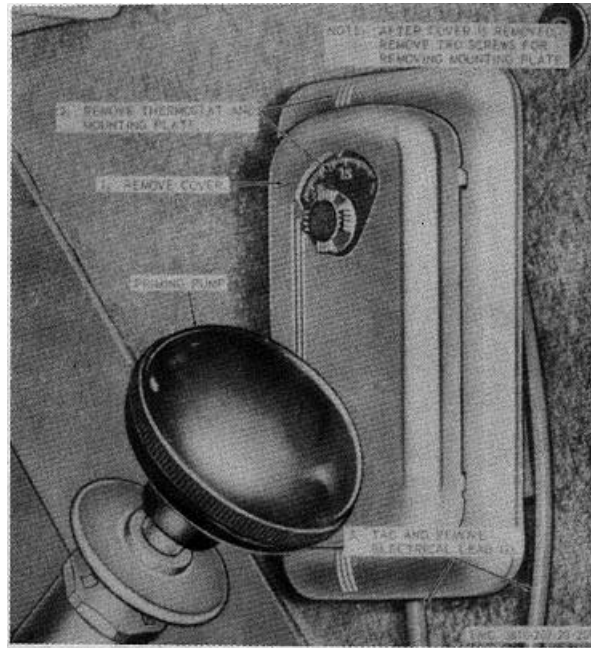
Figure 209. Thermostat, removal and installation.
